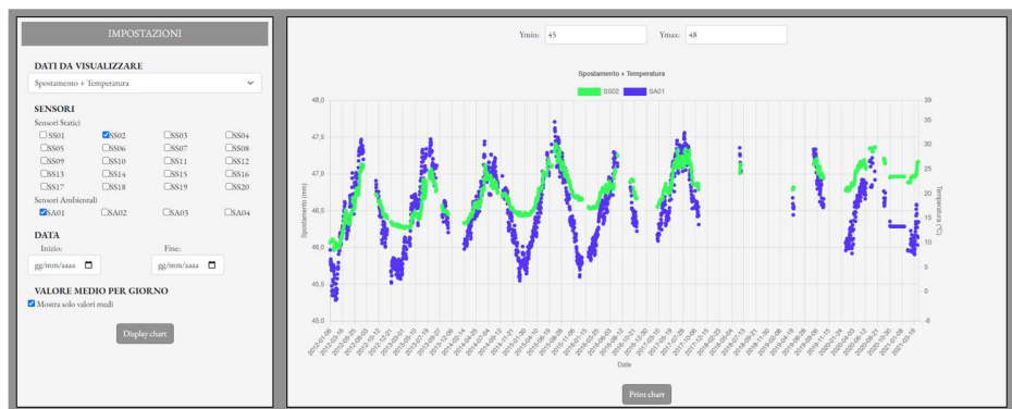
Figure 4. Example of graph generated by the web pages, selecting a static and an environmental sensor, no date and average value per day, from a minimum of 45 mm and a maximum of 48 mm.
