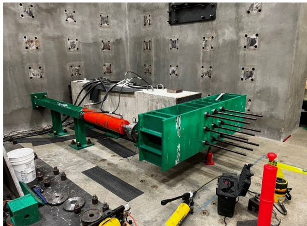
Figure 2: Trunnion beam's test configuration.
