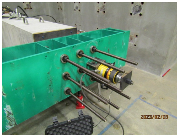
Figure 3: Trunnion rods' post-tensioning and load balancing prior to testing.
