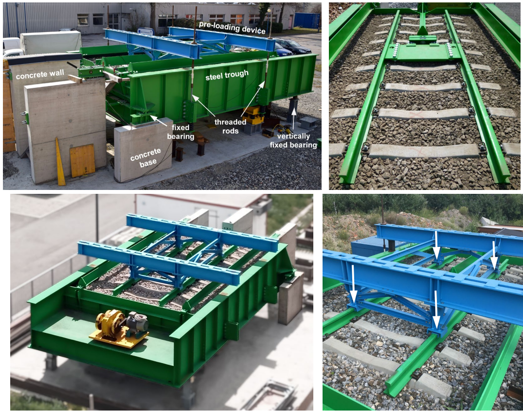
Figure 5. Large-scale test facility for isolated research of longitudinal track-bridge interaction (TBI) – top left: overview – top right: integrated section of ballast superstructure – bottom left: front view – bottom right: pre-loading device simulating two static axle loads of a train.
