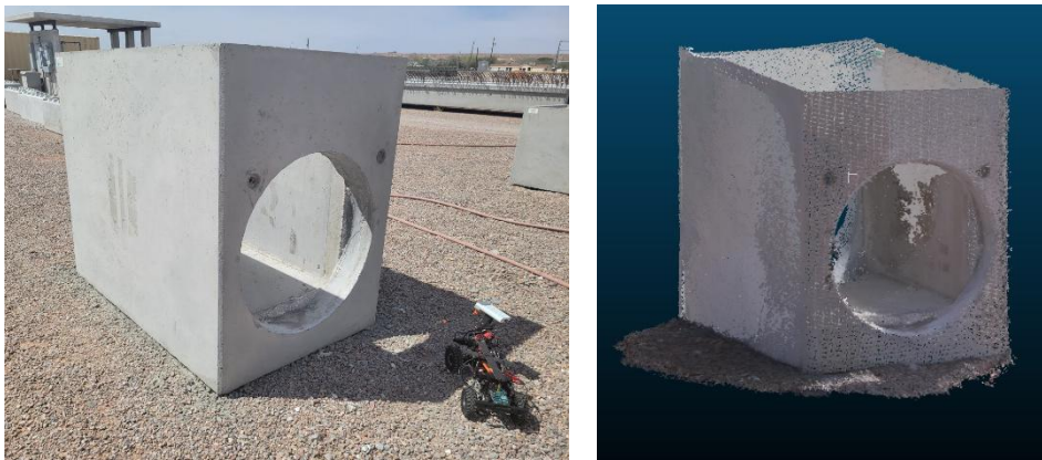
Figure 5: A catch basin in two forms, a physical concrete element (left) and its corresponding 3D point cloud model (right) from field testing.
