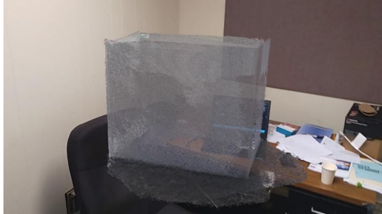
Figure 6: A holographic visualization of a catch basin created from 3D point cloud data, appearing as a three dimensional structure on a desk.
