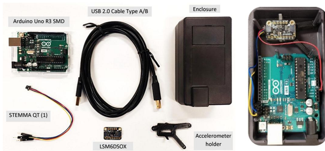
Figure 1. LEWIS1 Accelerometer components and assembly.
