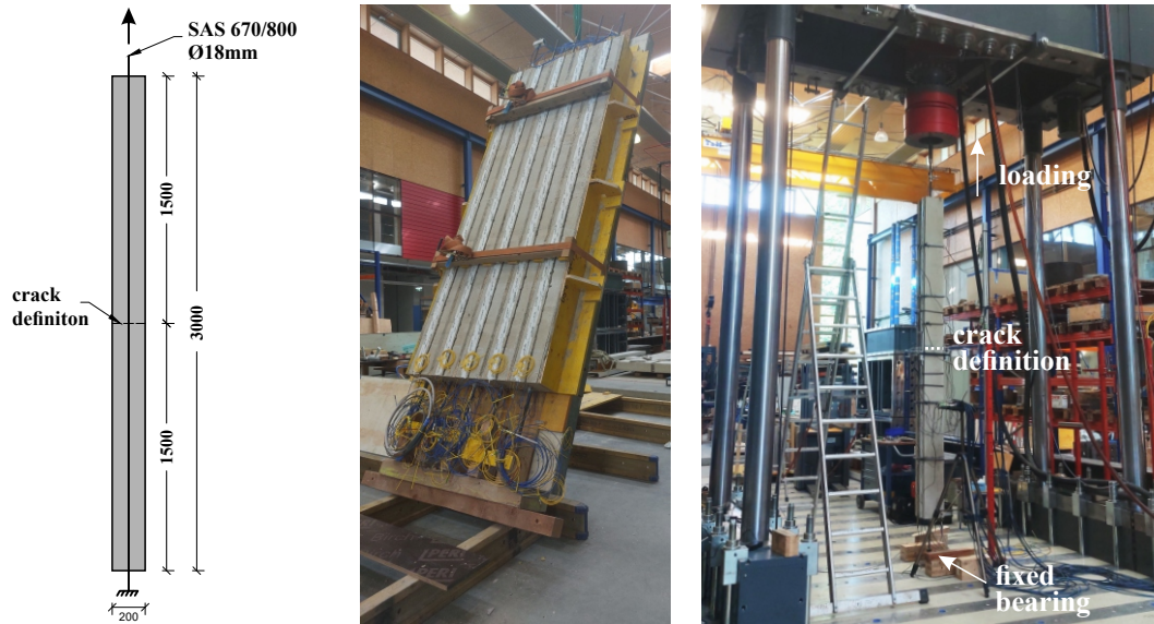
Figure 1. Laboratory test setup: Schematic representation (left), manufactured test specimens with applied DFOS cable (middle) and practical realization with one crack definition (right).
