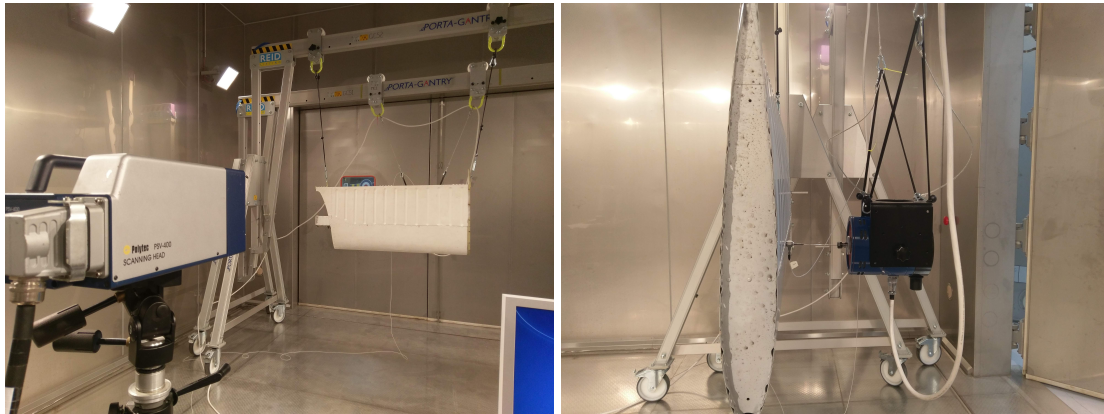
Figure 2. An example of a tailplane structure tested with a scanning laser vibrometer [12] (left). Shaker setup (right).
