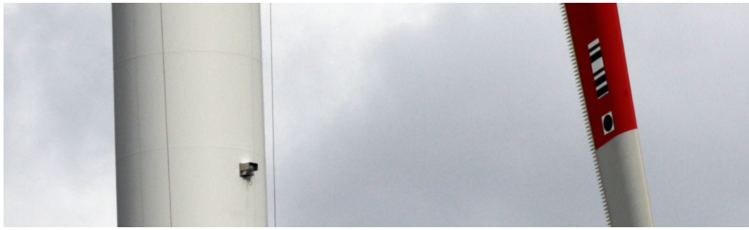
Figure 1. The sensor unit on the tower (left) and a rotor blade with barcode (right top) and AI marker (right bottom).
