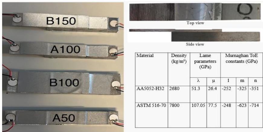
Figure 2. (a) The different specimens and their top and side view [15], and (b) show the properties of the different specimens.
