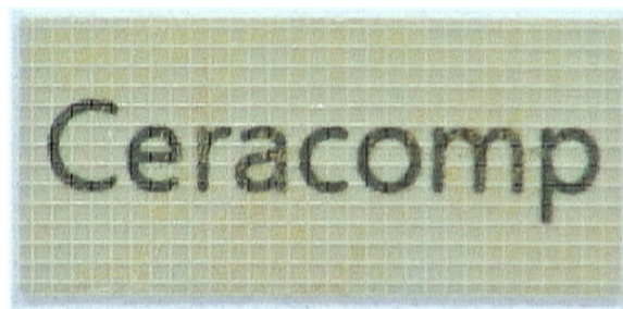
Fig. 5. Transparent 1-3 Single Crystal-Polymer Composite
