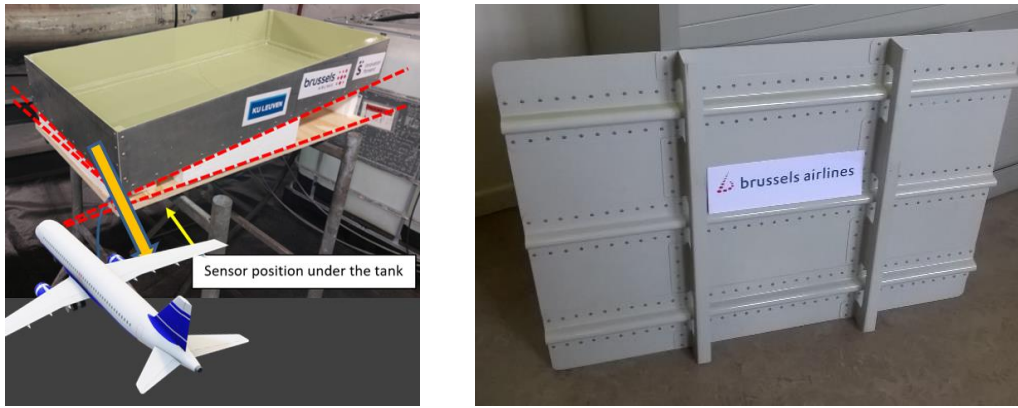
Figure 3. Left) Generic replica of a section of a fuel tank. The dashed red lines indicate the characteristic inclination of the wings (modelled on an A330), and the model aircraft schematically shows the analogous orientation of the underside of the tank section, so that its approximate position in relation to the wing profile can be assessed (the aircraft was taken from the MS Word 3D model), Right, replica of a fuselage panel.[9].
