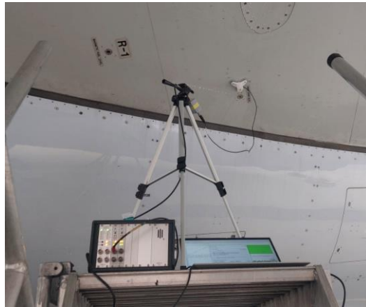
Figure 1. Setup for monitoring ice melting by acoustic emission sensors located close to the water drain valves at the wing sections (Airbus A330).
