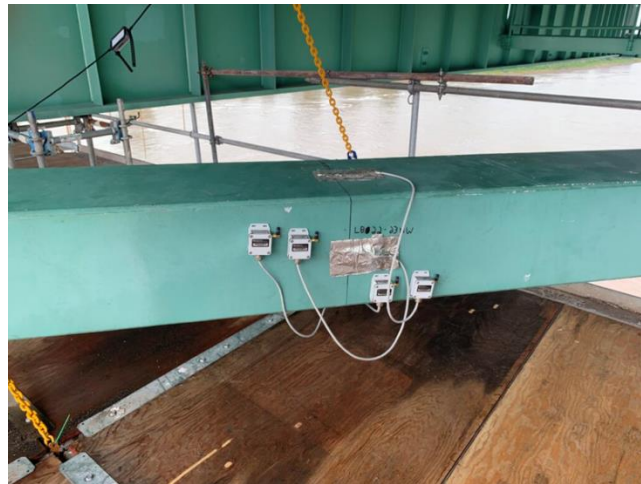
Figure 4. Installed wireless strain gauges SenSpot™ sensors on I-40 bridge
