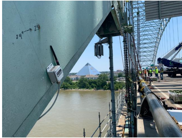
Figure 3. Examples of installed wireless strain gauge SenSpot™ sensors on I-40 bridge (the wireless unit with the antenna on the left side of the picture)
