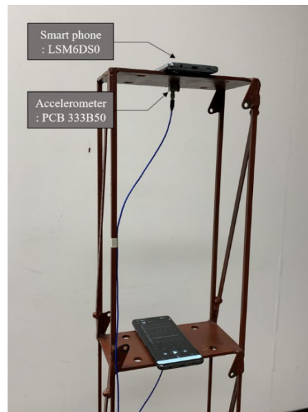
Figure 2. Photograph of steel frame and sensors.
