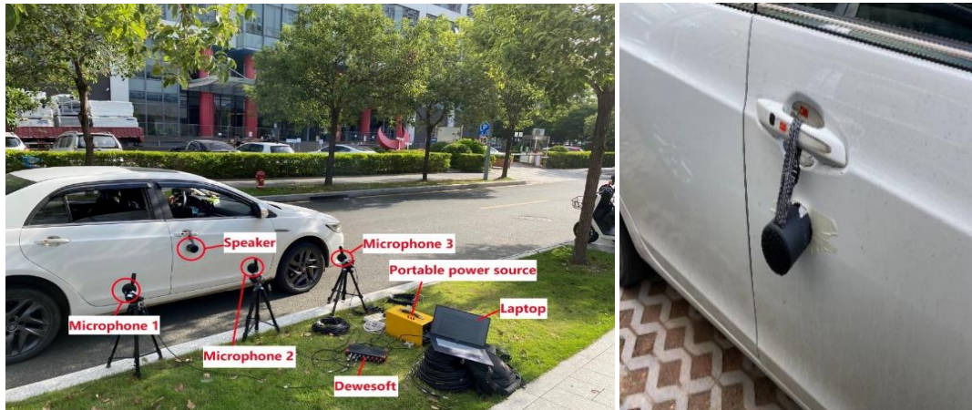
Figure 2. Field test of the simulated wayside acoustic train bearing fault diagnosis.
