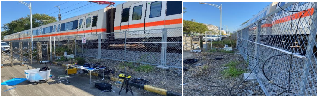
Figure 5. Field test of the trackside acoustic train bearing fault diagnosis.
