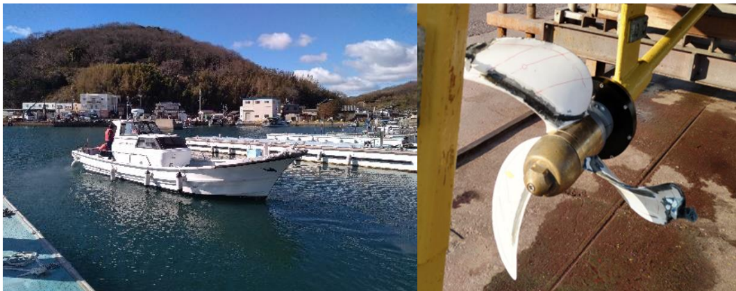
Figure 5. Leisure fishing boat (left) and CFRP propeller blades with embedded sensors and damage (right).
