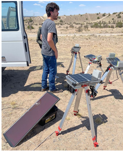
Figure 8. Components (LEWIS rainfall, sonar, and hotspot units) within a LEWIS network being prepped for deployment at a site.
