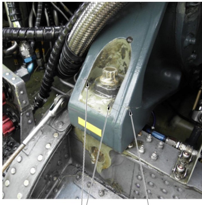
Figure 2: Cracked Main Gearbox attachment lug at R/H FS 290. Crack lines are marked. (Source: RNoAF)
