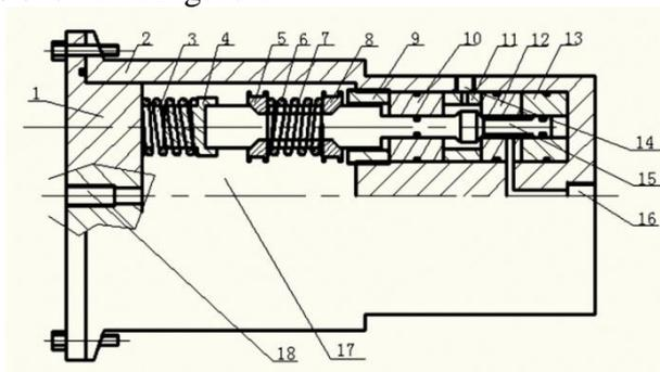
Figure 1. Diagram of sampling valve structure.
