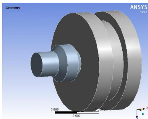
Figure 2. Valve head and valve seat sealing contact model diagram.
