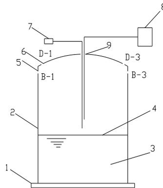
1. Electronic balance; 2. Tank wall; 3. N-hexane; 4. Floating deck; 5. Tank wall vent; 6. Tank top edge vent; 7. Anemometer; 8. Air bag; 9. Test window
