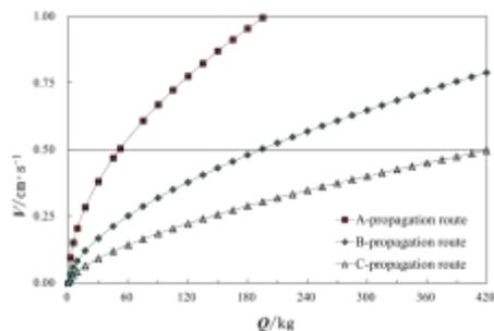
**Figure 5.** Relationship between the vibration velocities of different paths with variety explosive charges.
