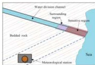
**Figure 4.** Schematic of the partition control for the blasting excavation.
