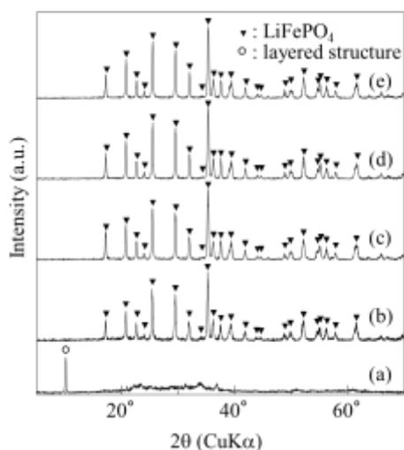
Figure 2. XRD patterns of the products synthesized by hydrothermal process at various temperature for 24h.
