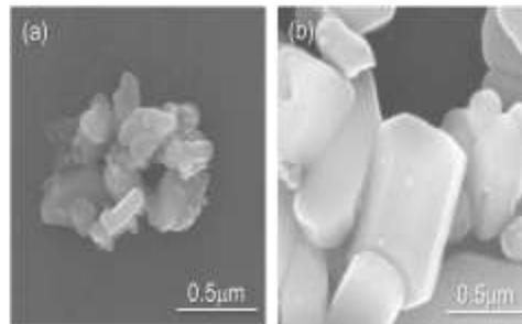
**Figure 5.** SEM images of the products synthesized by hydrothermal process at 473K for 1~72h. (a) 1h, and (b)72h.
