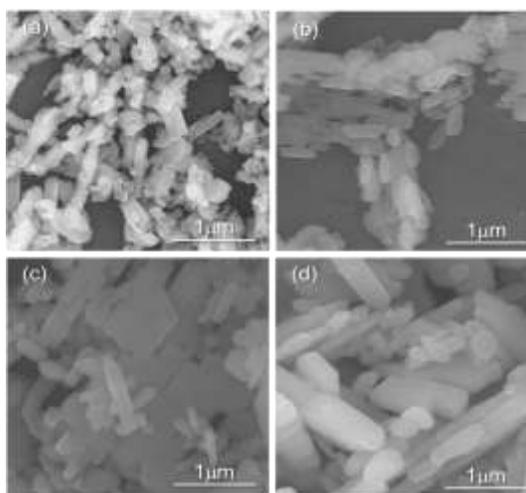
Figure 3. SEM images of the products synthesized by hydrothermal process at various temperature for 24h.
