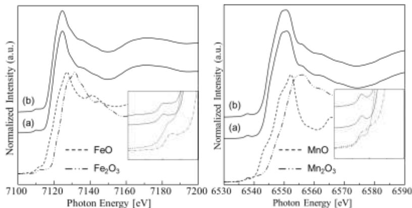
**Figure 8.** XANES spectra of the Mn added products synthesized by hydrothermal process (a)  $x=0$ , and (b)  $x=0.25$ .
