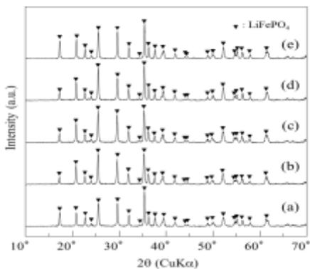
**Figure 4.** XRD patterns of the products synthesized by hydrothermal process at 473K for 1~72h. (a) 1h, (b)3h, (c)6h, (d)12h, and (e)72h
