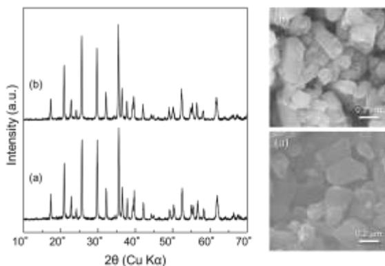
**Figure 6.** XRD patterns and SEM images of the Mn added products synthesized by hydrothermal process. (a)  $x=0$ , and (b)  $x=0.25$ .
