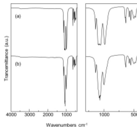
**Figure 7.** FTIR spectra of the Mn added products synthesized by hydrothermal process. (a)  $x=0$ , and (b)  $x=0.25$ .
