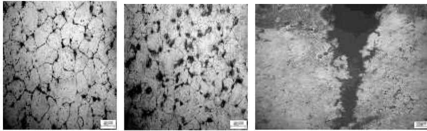
( a ) microstructure of the end ( b ) inclusions on the grain boundary ( c ) morphology of cracks
