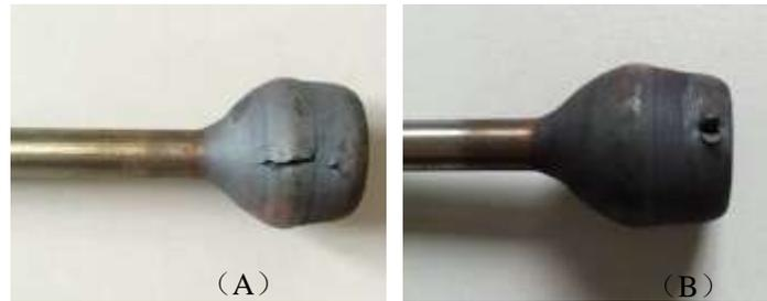
Figure 1. Inlet valve cracks of electrical upsetting.
