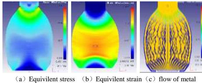
**Figure 6.** Scheme 2 simulation result.
