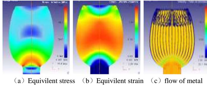
Figure 9. Scheme 5 simulation result.
