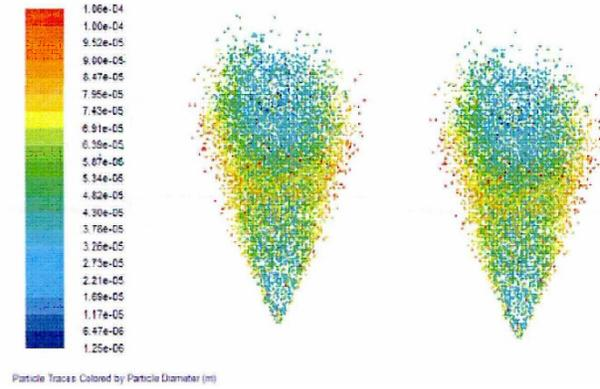
Figure 4. The spray particle size distribution.
