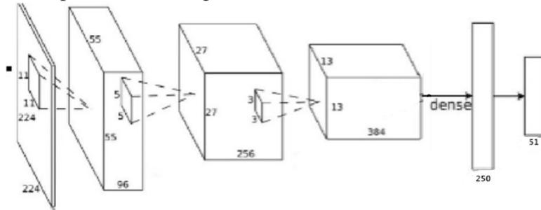
Figure 4. Convolutional neural network for depth feature.
