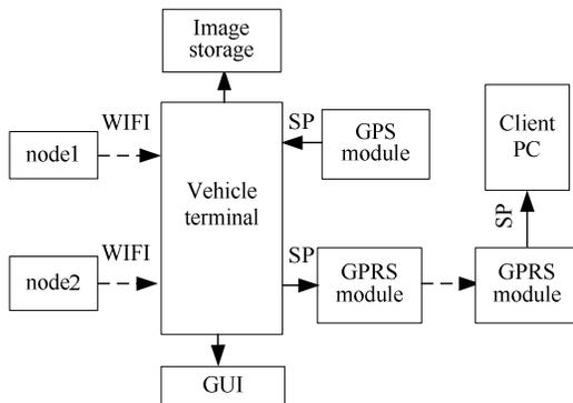
Figure 2. System hardware block diagram.
