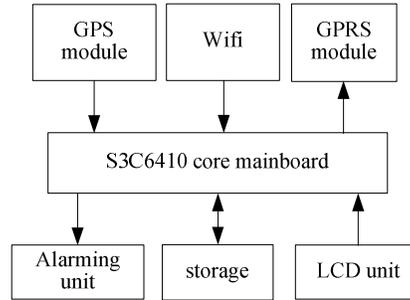
Figure 5. Vehicle monitoring terminal hardware block diagram.
