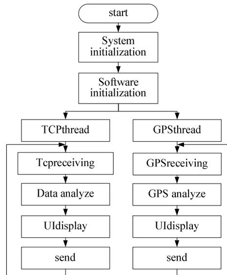
Figure 7. Vehicle monitoring terminal software flowchart.
