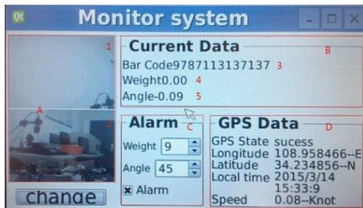
Figure 8. Vehicle monitoring terminal
