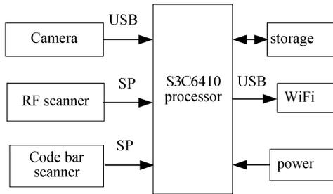
Figure 4. Data Acquisition Node two.
