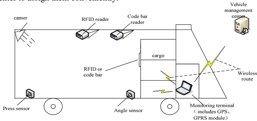
Figure 1. The diagrammatic sketch of logistic vehicle monitoring and management system
