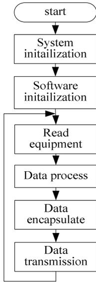
Figure 6. Data Acquisition Node software flowchart.
