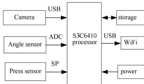
Figure 3. Data Acquisition Node one.
