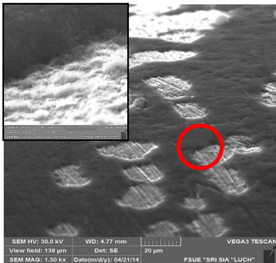
Figure 1. Nickel surface with coating from nanoparticles Al<sub>2</sub>O<sub>3</sub>.
