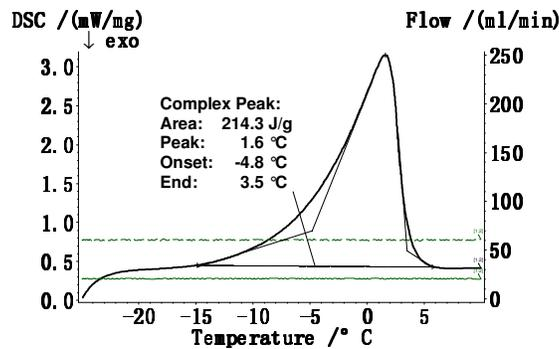
Figure 2. The DSC curve of mixture B in phase change process.
