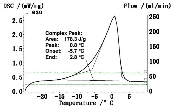
Figure 3. The DSC curve of mixture C in phase change process.
