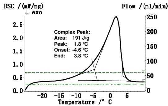
Figure 1. The DSC curve of mixture A in phase change process.
