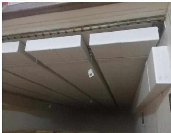
Figure 5. The concept sample of 20 feet refrigerator car with cold-hold plate.
